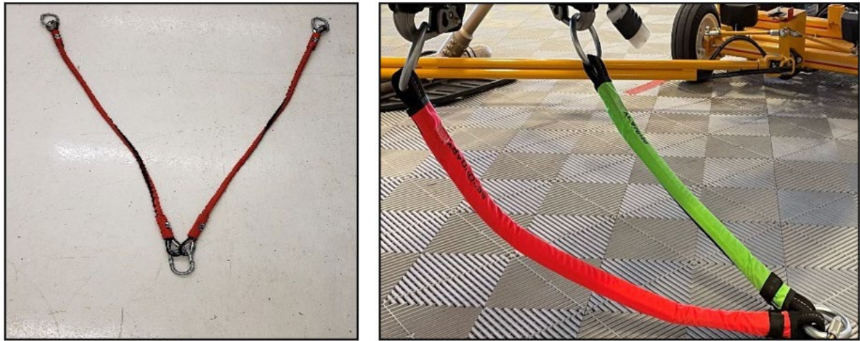
Figure 3-2 Left, Boost Y-Lanyard. Right, Onboard Systems Y-Rope.
